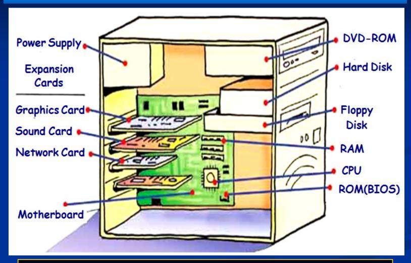
The most basic components inside central unit (case)
