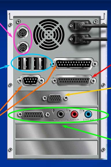
Parallel Port: older interface used to connect fast peripherals with high speed requirements (monitor, scanner). Today it has been replaced by USB. It is 8 times faster in data transmission than serial port.
